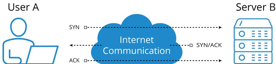
Figure 34. TCP/IP 3-way handshake
